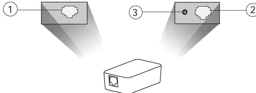
Port ①: Connect with the IP Phone EXT port or Expansion Module port (expansion module connected to the phone) through RJ12 cord.
